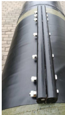
Tape and outer cover with closure flange and permanent bolt sets
